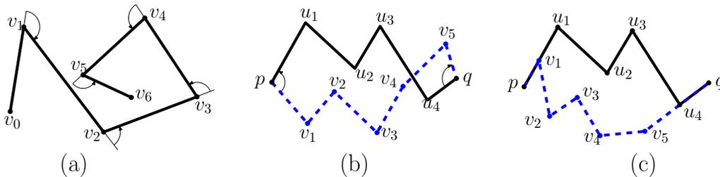
Figure 3: (a) The turning angles of a polygonal path. (b) Two crossing polygonal paths with the same turning angle between  $p$  and  $q$ . (c) Two noncrossing polygonal paths with the same turning angle between  $p$  and  $q$ .
